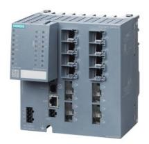
SCALANCE XM408-4C; managed modular IE switch; 8x 10/100/1000 Mbit/s RJ45; 4x 100/1000 Mbit/s ST-/SC- Pluggable as combo ports; in total 8 ports can be used; expandable to 24 ports electrical or optical; assembly: DIN rail/S7 mounting rail, PROFINET IO device; redundancy functions; office features (RSTP, VLAN, IGMP,..); C-plug in scope of delivery; Layer 3 with key plug available
