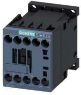
Power contactor, AC-3 12 A, 5.5 kW / 400 V 1 NC, 24 V DC with varistor integrated, 3-pole, size S00, screw terminals Upright mounting position
