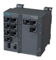
SCALANCE X310FE, managed plus IE switch, 10x 10/100 Mbit/s RJ45 ports, LED diagnostics, error-signaling contact with Select/set pushbutton, PROFINET IO Device, network management, integrated redundancy manager, Office features (RSTP, VLAN, IGMP,...) C-plug in scope of delivery
