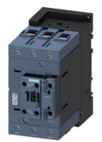
power contactor, AC-3 95 A, 45 kW / 400 V 1 NO + 1 NC, 110 V AC, 50 Hz Hz 120 V/60 Hz 3-pole, 3 NO, Size S3 screw terminal
