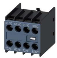
Auxiliary switch on the front, 4 NC Current path 1 NC, 1 NC, 1 NC, 1 NC for contactor relays Size S00 screw terminal 51/52, 61/62, 71/72, 81/82 Physically coded; only with contactor relays 3RH2140\* and 3RH2440\* can be combined (according to EN 50011)
