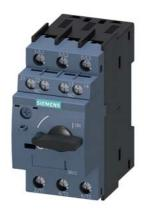
Circuit breaker size S00 for motor protection, CLASS 10 A-release 1.1...1.6 A N-release 21 A screw terminal Standard switching capacity with transverse auxiliary switches 1 NO+1 NC
