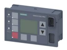
Operator panel with display for SIMOCODE pro V, installation in control cabinet door or front plate, can be plugged onto basic unit or extension modules, 7 LEDs for status display and 4 freely assignable keys for manual control, Color: titanium gray
