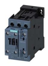
Contactor, 10 hp, 460 / 575 V, 1 NO + 1 NC, 24 V DC, 3-pole, Size S0 screw terminal
