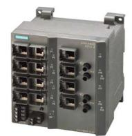
SCALANCE X212-2, managed IE switch, 12x 10/100 Mbit/s RJ45 ports, 2x 100 Mbit/s multimode BFOC, LED diagnostics, error-signaling contact with set button, redundant power supply, PROFINET IO device, network management, redundancy manager integrated, incl. electron. manual on CD-ROM, C-plug optional
