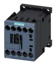
Coupling contactor relay, 4 NO, 24 V DC, 0.7  $\dots$  1.25\* US, with integrated diode, Size S00, screw terminal suitable for PLC outputs
