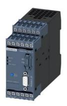
Basic unit SIMOCODE pro V PB PROFIBUS DP interface 12 Mbit/s, RS 485, 4I/3O freely parameterizable, Us: 110...240 V AC/DC, input for thermistor connection Monostable relay outputs, expandable by extension modules
