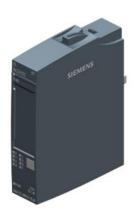
SIPLUS ET 200SP DI 8x24 V DC standard based on 6ES7131-6BF01-0BA0 with conformal coating, -40...+70 °C, digital input module, suitable for BU type A0, color code CC01, sink input, (PNP, sinking input), input type 3 (IEC 61131), input delay 0.05..20 ms module diagnostics for: short-circuit encoder supply, wire break, supply voltage
