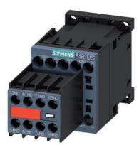
contactor relay, 7 NO + 1 NC, 110 V AC, 50 Hz / 120 V, 60 Hz, size S00, screw terminal, captive auxiliary switch
