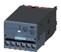
Solid-state time-delayed auxiliary switch OFF delay without control signal Relay 1 NC + 1 NO 24...240 V AC/DC Time range 0.05...100 s Can be snapped on at the front For 3RT2 S00-S3 contactors and 3RH2 S00 contactor relays Screw terminal Varistor for attenuation of the contactor coil integrated
