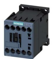
Contactor, AC-3, 7.5 KW / 400 V, 1 NO, 110 V AC, 50 Hz, 120 V, 60 Hz, 3-pole, Size S00 screw terminal
