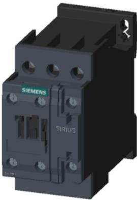
Power contactor, AC-3 38 A, 18.5 kW / 400 V 1 NO + 1 NC, 220 V AC 50 Hz, 240 V, 60 Hz 3-pole, Size S0, screw terminals
