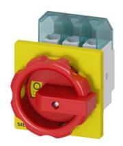
SENTRON, Switch disconnector 3LD, emergency switching-off switch, 3-pole, lu: 25 A, operating power / at AC-23 A 400 V: 9.5 kW, front-mounted, rotary operating mechanism, Red / yellow, 4-hole mounting of the handle
