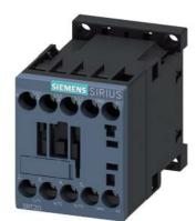
Power contactor, AC-3 12 A, 5.5 kW / 400 V 1 NO, 110 V AC, 50 Hz, 120 V 60 Hz, 3-pole, Size S00 screw terminal
