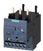
Overload relay 6...25 A Electronic For motor protection Size S0, Class 20E Contactor mounting Main circuit: Screw Auxiliary circuit: Screw Manual-Automatic-Reset
