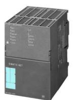
Communications processor CP 343-1 Advanced for connection of SIMATIC S7-300 CPU to Industrial Ethernet: PROFINET IO controller a./o. IO device; RT and IRT, MRP, PROFINET CBA; TCP/IP, ISO, UDP, S7 comm., S5-compat. communication (SEND/RECEIVE) with Fetch/Write RFC1006, Multicast Diagnostic extension, SNMP, DHCP, FTP client/server, email, Gigabit-SS1X RJ45 (10/100/1000); PROFINET interface 2x RJ45 (10/100 Mbit); PROFINET CBA; firewall/VPN; PROFIenergy
