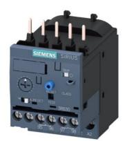
Overload relay 3...12 A Electronic For motor protection Size S00, Class 10E Contactor mounting Main circuit: Screw Auxiliary circuit: Screw Manual-Automatic-Reset
