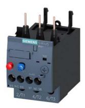
Overload relay 11...16 A Thermal For motor protection Size S0, Class 10 Contactor mounting Main circuit: Screw Auxiliary circuit: Screw Manual-Automatic-Reset
