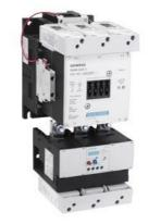
Non-reversing motor starter Size 5 Three phase full voltage Solid-state overload relay OLRelay amp range 55-250A 110-127V 50-60HZ/DC coil Combination type No enclosure
