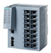
SCALANCE XC216 managed Layer 2 IE switch; IEC 62443-4-2 certified; 16x 10/100 Mbps RJ45 ports; 1x console port, diagnostics LED; redundant power supply; temp. range -40 °C to +70 °C; mounting: DIN rail/S7 mounting rail/wall Office redundancy functions features (RSTP, VLAN,...); PROFINET IO device; Ethernet/IP-compliant; C-plug slot;
