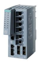
SCALANCE XC206-2 managed Layer 2 IE switch; IEC 62443-4-2 certified; 6x 10/100 Mbps RJ45 ports; 2x 100 Mbps SC ports; 1x console port; diagnostics LED; redundant power supply; temp. range -40 °C to +70 °C; mounting: DIN rail/S7 mounting rail/wall; redundancy functions; Office features (RSTP, VLAN,...); PROFINET IO device Ethernet/IP-compliant C-plug slot
