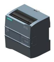
SIMATIC S7-1200, CPU 1212C, compact CPU, DC/DC/relay, onboard I/O: 8 DI 24 V DC; 6 DO relay 2 A; 2 AI 0-10 V DC, Power supply: DC 20.4-28.8V DC, Program/data memory 50 KB
