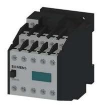
Contactor relay, 91E, EN 50011, 9 NO + 1 NC, screw terminal, AC operation, 24 V AC 50/60 Hz
