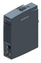
SIMATIC ET 200SP, digital output module, DQ 16x 24VDC/0.5A Basic, Pack quantity: 1 unit, suitable for BU type A0, Color code CC00, Module diagnostics
