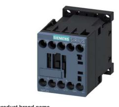
power contactor, AC-3 12 A, 5.5 kW / 400 V 1 NC, 24 V DC 3-pole, Size S00 screw terminal
