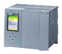
SIMATIC S7-1500TF, CPU 1516TF-3 PN/DP, Central processing unit with 1.5 MB RAM for program and 5 MB for data, 1st interface: PROFINET IRT with 2-port switch, 2nd interface, Ethernet, 3rd interface, PROFIBUS, 10 ns bit performance, SIMATIC Memory Card required
