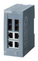
SCALANCE XB004-2 unmanaged Industrial Ethernet Switch for 10/100 Mbit/s; for setting up small star and line topologies; LED diagnostics, IP20, 24V DC power supply, with 4x 10/100 Mbit/s twisted pair ports with RJ45 sockets; 2x 100 Mbit/s multimode glass FOC port with SC socket; Manual available as a download
