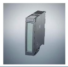
SIMATIC S7-1500, digital output module DQ 16x230 V AC/1 A ST; TRIAC; 16 channels in groups of 2; 2 A per group; Substitute value: Front connector (screw terminals or push-in) to be ordered separately
