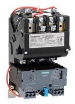
Non-reversing motor starter Size 1 Three phase full voltage Solid-state overload relay OLRelay amp range 5.5-22A 24VAC 50-60HZ coil Combination type No enclosure
