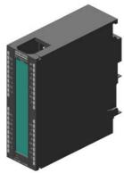
SIMATIC S7/PCS7, digital output SM 322, 16 DO; 24 V DC / 0.5 A, diagnostics-capable, wire break detection with 0 and 1 signal, 1 x 40-pole, interface IM 153-X HF required
