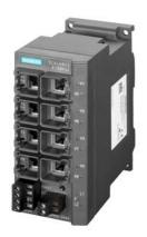
SCALANCE X108PoE unmanaged IE switch, 2x 10/100 Mbit/s RJ45 Power-over-Ethernet ports and 6x 10/100 Mbit/s RJ45 ports, LED diagnostics, error signaling contact with set button, Redundant power supply Manual available as a download
