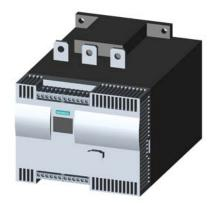
SIRIUS soft starter Values at 500 V, 40 °C standard: 203 A, 132 kW Inside-delta: 352 A, 250 kW 400-600 V AC, 230 V AC Screw terminals !!! Phased-out product !!! Successor is SIRIUS 3RW5, Preferred successor type is >>3RW5543-6HA16<<
