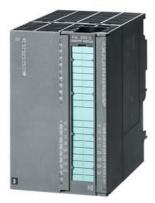
SIPLUS S7-300 FM350-2 8 channels for medial exposure with conformal coating based on 6ES7350-2AH01-0AE0 . Counter module FM 350-2, 8 channels, 20 kHz, 24 V encoder for counting, frequency measurement, speed measurement, period duration measurement, dosing incl. configuration package and Electronic documentation on CD-ROM
