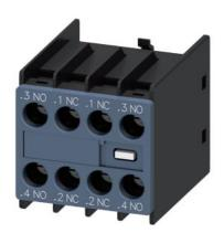
Auxiliary switch on the front, 2 NO + 2 NC Current path 1 NO, 1 NC, 1 NC, 1 NO for 3RH and 3RT screw terminal .3/.4, .1/.2, .1/.2, .3/.4
