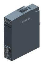
SIPLUS ET 200SP DQ 16x24VDC/0,5A ST based on 6ES7132-6BH01-0BA0 with conformal coating, -40...+70 °C, digital output module, suitable for BU type A0, color code CC00, module diagnostics
