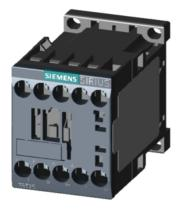
Power contactor, AC-3 16 A, 7.5 kW, 400 V 2 NO + 2 NC 230 V AC, 50/60 Hz 4-pole Size S00 Screw terminal
