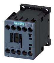
Power contactor, AC-3 9 A, 4 kW / 400 V 1 NO, 110 V AC, 50 Hz, 120 V 60 Hz, 3-pole, Size S00 screw terminal
