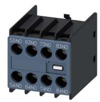
Auxiliary switch on the front, 4 NO Current path 1 NO, 1 NO, 1 NO, 1 NO for contactor relays Size S00 screw terminal 53/54, 63/64, 73/74, 83/84 for 3RH2140/3RH2440 acc. to EN 50011 Physically coded; only with contactor relays 3RH2140\* and 3RH2440\* can be combined (according to EN 50011)
