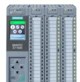
SIMATIC S7-1500 Compact CPU CPU 1512C-1 PN, central processing unit with working memory 250 KB for program and 1 MB for data, 32 digital inputs, 32 digital outputs, 5 analog inputs, 2 analog outputs, 6 high speed counters, 4 high speed outputs for PTO/PWM/frequency output 1. interface: PROFINET IRT with 2 port switch, 48 NS bit-performance, incl. front connector push-in, SIMATIC memory card necessary
