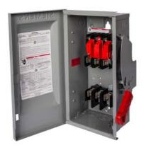
Siemens Low Voltage Circuit Protection Heavy Duty Safety Switches. Type: ENCLOSED, SAFETY SWITCH Std: UL V. Rating: 600V A. Rating: 200A Wattage: 3W No. Of Poles: 3P F. Rating: 60Hz Action: SINGLE THROW Material: 304SS Enclosure: TYPE 3R. 2-3 point mounting holes. O. Cycles: 8000 O. Temperature: (-20F-120F) AMBIENT TEMPERATURE Environmental Conditions: OUTDOOR
