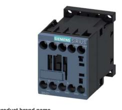
Coupling contactor relay, 3 NO + 1 NC, 24 V DC, 0.7  $\dots$  1.25\* US, with integrated diode, Size S00, screw terminal suitable for PLC outputs
