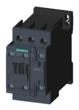
power contactor, AC-3 12 A, 5.5 kW / 400 V 1 NO + 1 NC, 110 V AC, 50 Hz 120 V, 60 Hz, 3-pole Size S0, screw terminal
