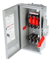
Siemens Low Voltage Circuit Protection Heavy Duty Safety Switches. Type: ENCLOSED, SAFETY SWITCH Std: UL V. Rating: 600V A. Rating: 30 A Wattage: 4W No. Of Poles: 3P F. Rating: 60Hz Action: SINGLE THROW Material: 304SS Enclosure: TYPE 3R. 2-3 point mounting holes. O. Cycles: 10000 O. Temperature: (-20F-120F) AMBIENT TEMPERATURE Environmental Conditions: OUTDOOR
