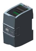
SIPLUS S7-1200 SM 1231 4 Al 13 bits for medial exposure with conformal coating based on 6ES7231-4HD32-0XB0 . Analog input, 4 Al, +/-10 V, +/-5 V, +/-2.5 V, or 0-20 mA 12-bit+ sign bit (13 bit ADC)
