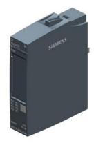
SIMATIC ET 200SP, Digital input module, DI 8x 24V DC SRC BA, type 1 (IEC 61131), source Input (NPN, M-reading) Packing unit: 1 piece, fits to BU-type A0, Colour Code CC02, input delay time 0,05..20ms, module diagnostics for: supply voltage
