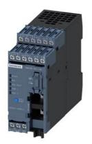
Basic unit SIMOCODE pro V PN, Ethernet/PROFINET IO, PN system redundancy, OPC UA server, Web server, transmission rate 100 Mbps, 2 x bus connection via RJ45, 4l/3O freely parameterizable, Us: 110...240 V AC/DC, input for thermistor connection Monostable relay outputs, expandable by extension modules
